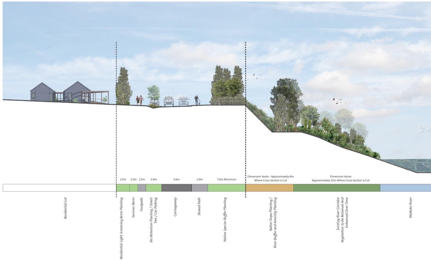
--- Northern River Road Cross Section 1:250 @ A3
